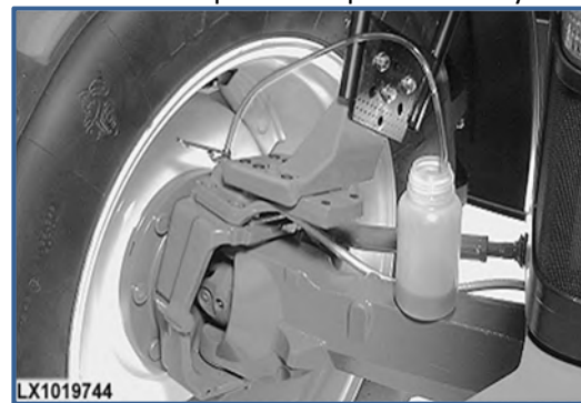
Fig 64: Bleeding of the front brakes (JD, 2018)
