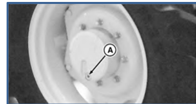
Fig 71: Front wheel hub drain- and fill-plug (JD, 2018)
