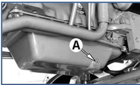
Fig 25: Drain plug of the crankcase (JD, 2018)
