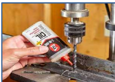
Fig 9: Lubricating the drill to extend its longevity (Wikipedia, 2018)
