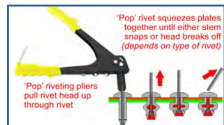
Fig 12 : Riveting sheet metal (Wikipedia,
