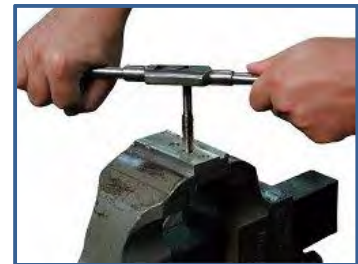
Fig 11 : Cutting internal thread with a tap (Wikipedia, 2018)
