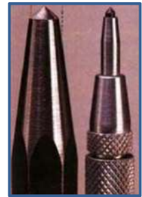
Fig 7 : A centre punch (left) and scribe (right) (Wikipedia, 2018)
